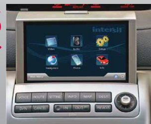
Intersil's proprietary SPI OSD engine allows for a low cost bit-map based OSD capability.
