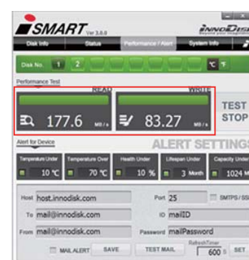
Performance/Alert page can show any installed disk's R/W performance
